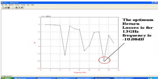
Fig. 5 Return Loss Vs Frequency (in GHz)
