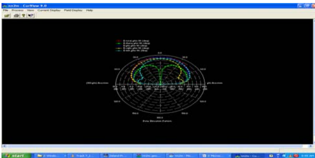
Fig. 18 Elevation Pattern of E Total, E Right, E Left, E Theta, E Phi at \Phi=90 (deg)
